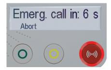
Example: The user recognises the remaining pre-alarm time and can cancel the call by pressing the green button.
